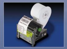
Thermal Printer TG 2460 II. Paper width: 60 mm. Printing speed: 120 mm/sec. Autocutter and static presenter. Anti paper-jam. USB interface.
