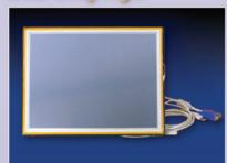
15" LCD TFT chassis. Resolution: 1024 x 768. Brightness 250 or 1500 cd/m2 optional. Contrast 400:1. Analog input. Touchscreen optional.
