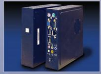
Industrial computer MSI. Suitable for difficult outdoor applications. Intel Mobile processor. 1 GB RAM. 80 GB HD. Size: 180(H) x 43(B) x 180(T) mm.
